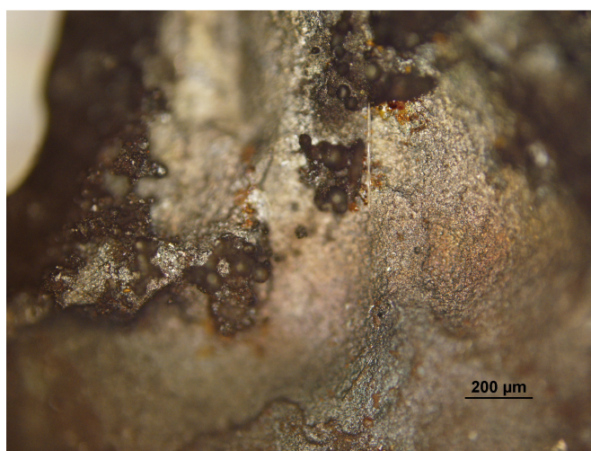
Figure 3- Optic microscope photograph of the filter. Orange colored zones (indicated) and brilliant streaks can be observed (10X)
