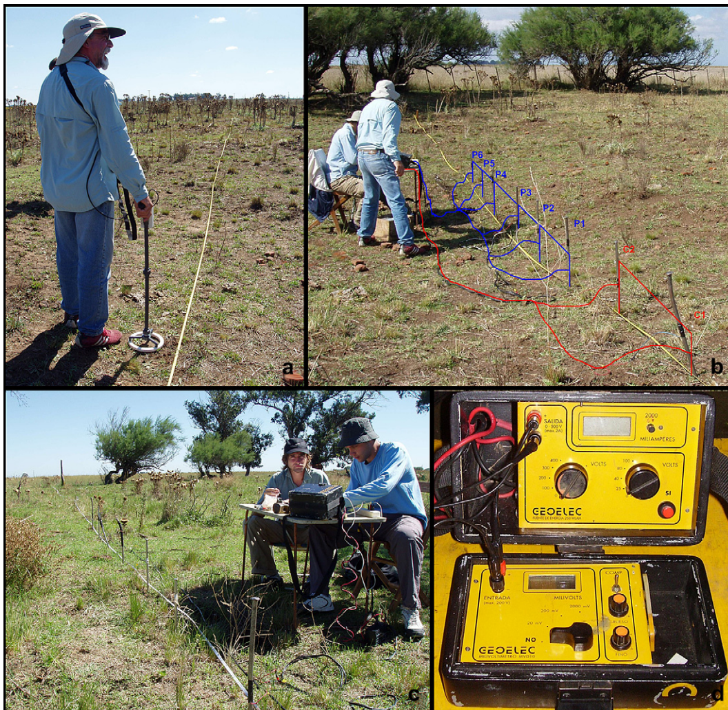
Fig. 4. Geophysical survey: equipment and devices. a. Magnetic Susceptibility meter b. Dipole device installation. c. Measure resistivity. d. Resistivity Meter System manufactured at Facultad de Ciencias Astronómicas y Geofísicas. Universidad Nacional de La Plata.
