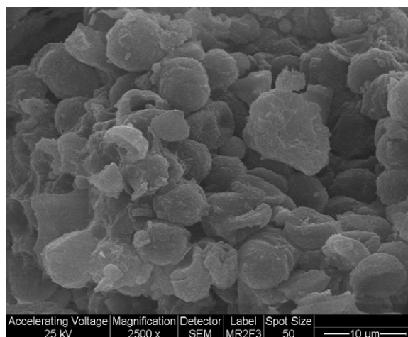
Fig. 3. SEM photomicrograph. Marble of the pre-intervention Rufina Cambaceres tombstone. Fungal microcolonies are observed.
