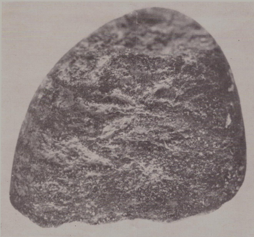
FIG. 12.—Photograph of a fragment of tuff showing the bedding planes, corresponding to measurements in table 1. Magnification 1\frac{1}{3} .
